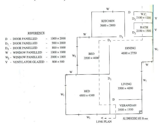
2. Draw the plan, section and elevation of given line daigram for a poposed primary health centre: assume the necessary data suitably.
