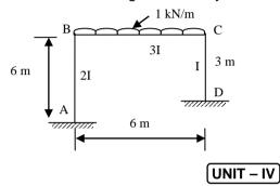
Analyze the continuous beam shown in figure below by matrix flexibility method and draw the bending moment diagram.
