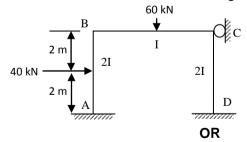
Analyze the portal frame shown in figure below by moment distribution method. The relative moment of inertia value for each member is indicated in the figure below. Sketch the bending moment diagram.
