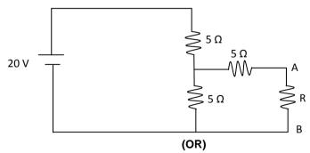
4 Calculate the open circuit impedance parameters for the resistor T-network shown in figure below.
