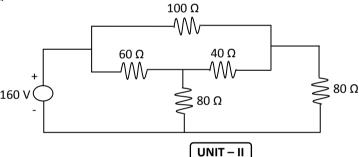
3 State maximum power transfer theorem. Find the value of R<sub>eq</sub> and determine maximum power to R for the given network.
