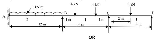
7 Analyze the frame shown in figure below by Kani's method.
